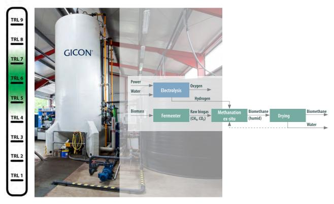
Since 2015, GICON® engineers have been working on the production of biomethane from hydrogen and carbon dioxide in so-called trickle bed reactors. The aim is to store renewable energy at peak loads in the power grid via the electrolysis of hydrogen and subsequent methanization.
