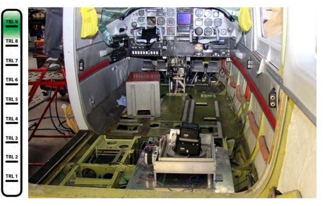
In the field of ornithological monitoring and analysis, GICON® can employ the Digital Aerial Imagery System by IfAÖ (DAISI), a tandem camera system developed in cooperation with the University of Rostock, which is aligned vertically to the observation area in an airplane and allows a ground resolution of 2 cm. Project applications of the photo flights have shown that with the DAISI system, an up to 98 percent higher accuracy is possible for species counts when compared to an observation flight.
