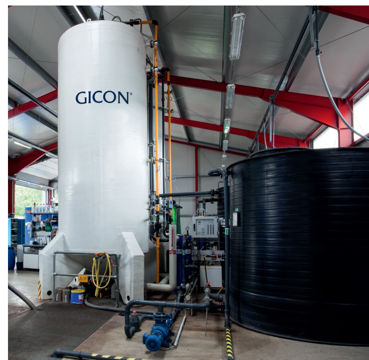
10 m 3 trickle bed reactor
