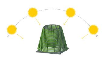
The core of the GICON<sup>®</sup> photobioreactor is the flexible silicone-based tubing system as a result of the success-ful cooperation between GICON<sup>®</sup> and Wacker Chemie AG. The highly transparent ELASTOSIL<sup>®</sup> silicone rubber and innovative double wall system provide a very convincing a solution for indoor and outdoor use.
