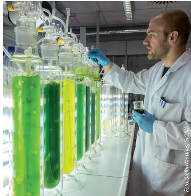
Microalgae cultivation using bubble column reactor in the laboratory.
