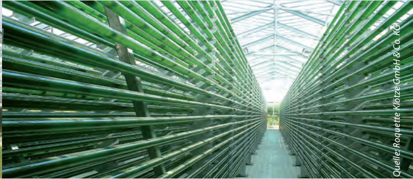
World's first and largest tubular production facility for micro-algae in Klötze, planned and built by GICON.
