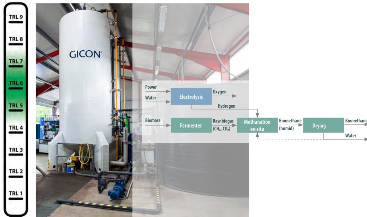
Since 2015, GICON® engineers have been working on the production of biomethane from hydrogen and carbon dioxide in so-called trickle bed reactors. The aim is to store renewable energy at peak loads in the power grid via the electrolysis of hydrogen and subsequent methanization. Trickle bed reactors can be used as supplementary systems for biogas/wastewater gas plants and power plants.
